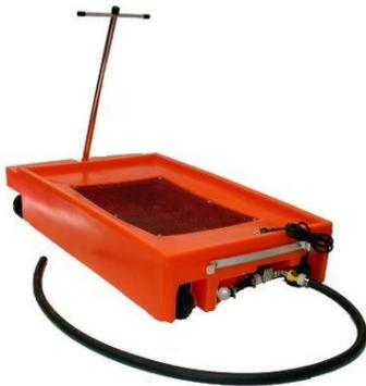
Low Boy Oil Drain with evacuation kit. Heavy duty polyethylene with wire screen. Translucent body for view of fluid level. 17 gallons. Four lubricated casters recessed into body.
