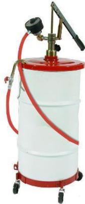
Gear Lube Pump - fits 120 lb. open head drums. Includes pump, drum cover, 5' (longer hoses not recommended) of medium pressure oil hose, non-drip curved discharge nozzle, MODEL 1500 universal pint meter, and MODEL 120-S drum dolly.
