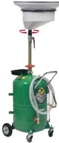
Adjustable Waste Oil Drain. 17 Gallon Capacity.
