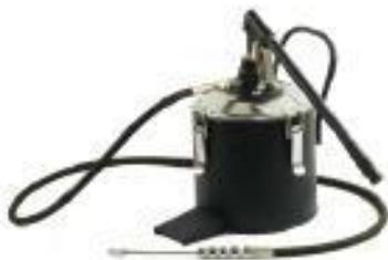
Hand pump for dispensing grease from 25 to 50-lb pails. Includes 22-lb fully enclosed container. Heavy duty cast iron construction. Includes spring loaded follower plate. Easy to carry handle.
