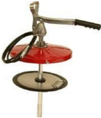
Grease Pump - hand operated grease pump for full open head pails up to 6-½ gallon size. Includes pump, cover, plastic handgrip, carrying handle, follower plate, 6-foot high-pressure hose, and MODEL 28 coupler.
