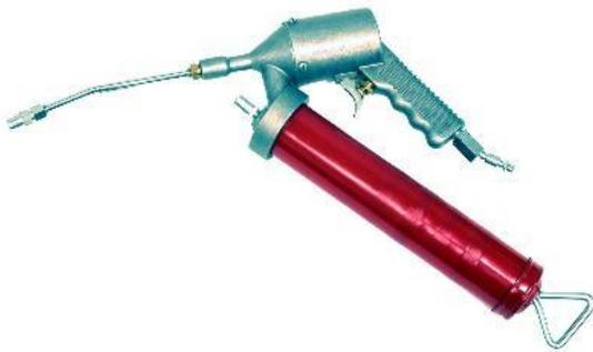
Single Shot Air operated pistol grip grease gun. 40:1 pressure ratio. Maximum pressure 4,000 PSI. 75 to 100 psi inlet pressure. Delivers .60 oz. per 40 strokes. Heavy duty aluminum die cast head with bulk loader valve. Internal bore precision honed for rapid action. Single shot operation.
