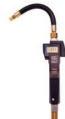
Digital meter for dispensing in pints, quarts, liters, or gallons. Totalizes in gallons or liters. Safety lock to prevent accidental operation. Cover and trigger are impact resistant plastic. 2 AAA batteries.
