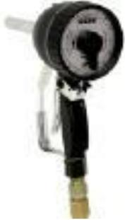
Quart Meter. Preset 1 to 16 quarts. Totalizes in U.S. quarts. Automatically shuts off at pre-selected quantity. Includes MODEL 1101 swivel connector and MODEL 1340 automatic non-drip rigid nozzle for motor oils.
