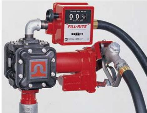
13 GPM. ¼ horsepower motor for ethylene glycol, diesel, fuel, grease, hydraulic oil, motor oil, and water. 110 volt or 12 volt.
