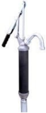
Barrel Pump - fits 15 through 55-gallon drums with 2" bung opening. Has a zinc die-cast piston with two brass rings, steel telescoping tube assembly, Buna N Seals, plastic handle grip, and curved discharge spout with garden hose threads. Dispenses approximately 1 pint per stroke. Has adjusting nut on bung threads.
