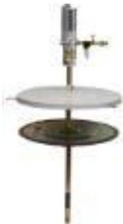
65:1 Grease pump system. Includes pump, drum cover, follower plate, air line filter, needle valve, and quick connects. Used to dispense grease from 400-lb. Open head drum.
